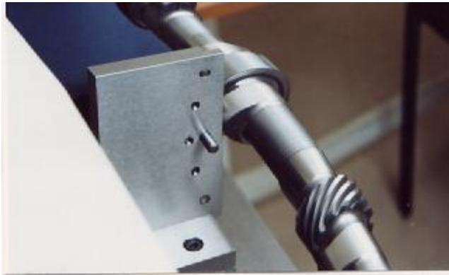
The requirement to measure with flat and radius followers has dictated a universal adaptor arrangement to suit various diameter roller inserts are available.
