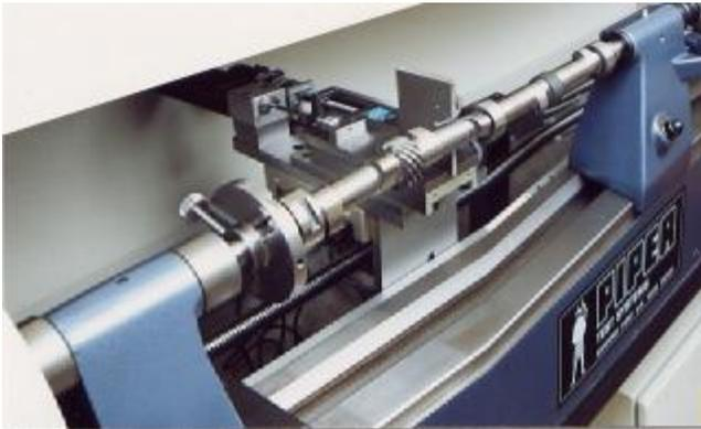
The adaptation of high quality tool room products has enabled a cost effective package to be created. Cam shaft up to 915mm between centres and with a swing diameter of 305mm can be accommodated.
