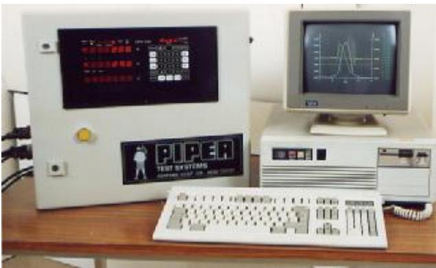
Piper has developed a user friendly software combination utilising their cam shaft design and manufacturing expertise to give a comprehensive monitoring and recording package. 'X' coordinates which are required for repeatable follower/lobe position are stored in files and are easy to retrieve.
